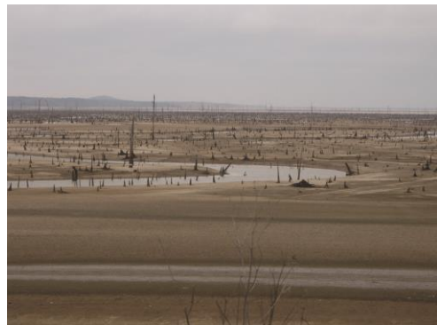
Figure 7.4. Drawdown in shallow Grenada Lake, Mississippi, showing desert-like mudflat areas in the regulated zone. U.S. Army Corps of Engineers, Vicksburg District.
