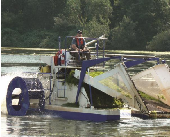
Figure 11.7. An aquatic plant harvester on Fairview Lake reservoir, Oregon, working to remove excessive underwater plant growth. Photo credit: B. Greene, The Oregonian .
