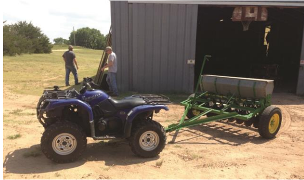
Figure 11.13. A drill seeder positions seeds in the mudflats at the proper depth and covers them, preventing predation by birds and improving germination rate over seed broadcasting. Photo credit: M. Lashley, Mississippi State University.
